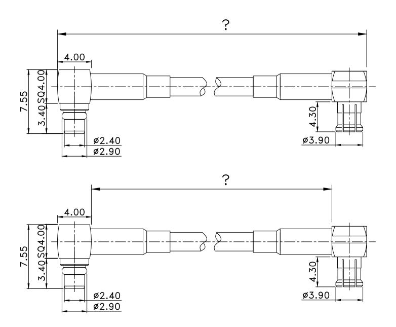
Customer Drawing (connectors excluded) <1M Customer Drawing (connectors included) >1M
