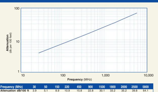
Calculate Attenuation = (0.709140) • √FMHz + (0.001740) • FMHz (interactive calculator available at http://www.timesmicrowave/telecom)
